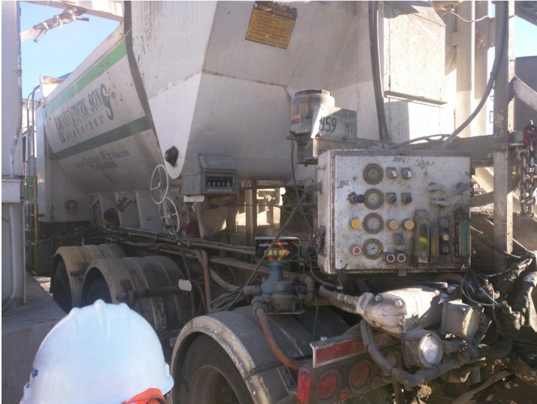
Figure 1 - Controls of Volumetric Mixer.
