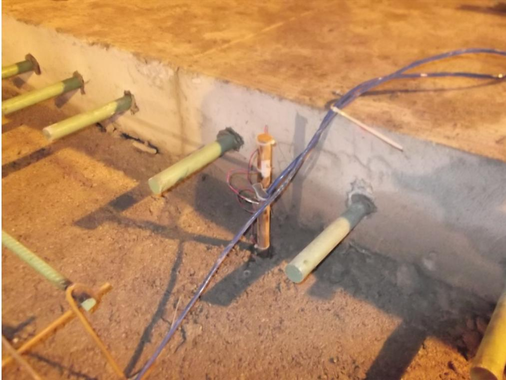
Fig. 27 – Layout of thermocouples at patch edge (patch 3).
